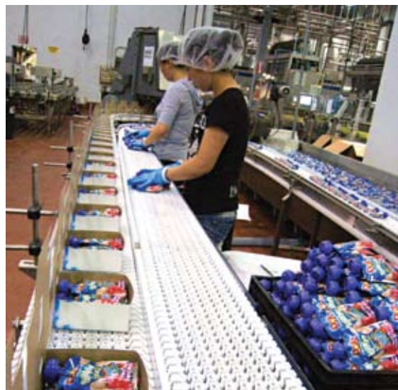
Before packing pouches into cartons using a special inserting pattern, workers straighten the pouches. This improves pouch presentation in the cartons’ windows.
