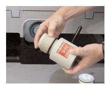
Thread 2" BSP pusher/cutter adapter to V50 gate valve.
