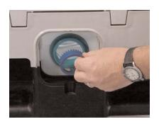
Flip crown cutter 180° and put back into fitment.
