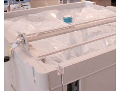
Place winder on opposite side of dispense location.
